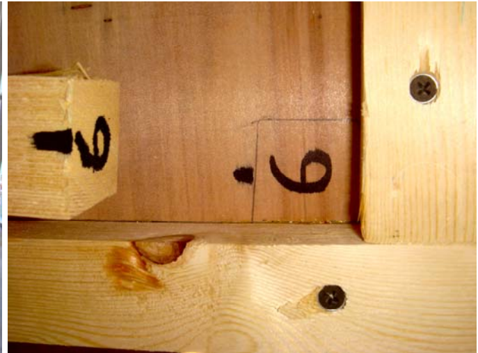
Fig. 11 – Each leg is numbered for reassembly.
