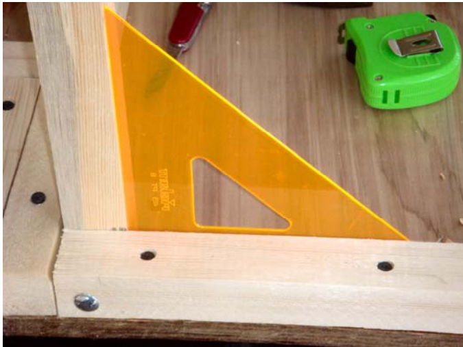
Fig. 12 – A triangle insures leg is square to the table top.
