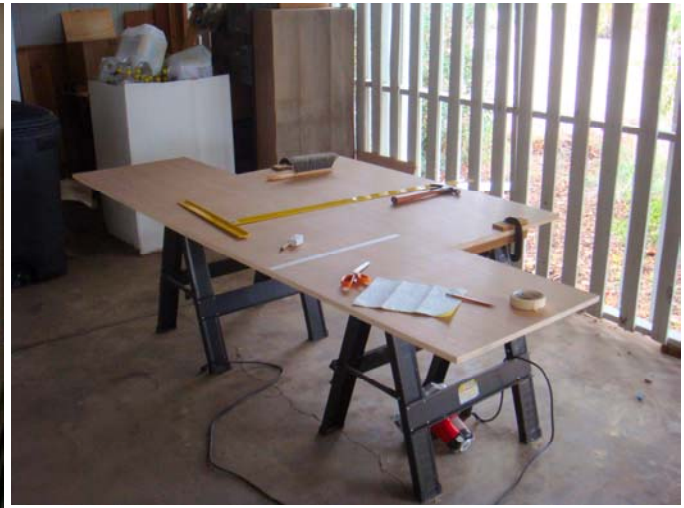
Fig. 7 – Masking tape is applied to the table for cutting.
