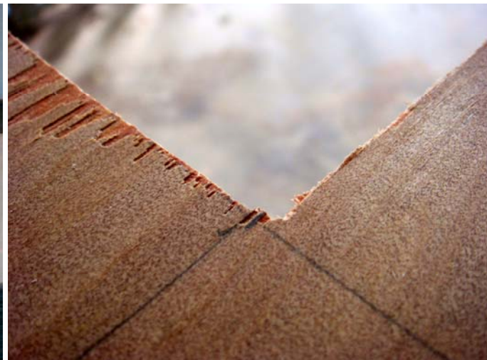
Fig. 9 – Left cut without tape, right cut with tape.
