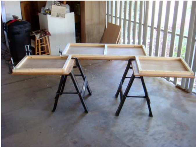
Fig. 10 – Gluing and screwing the 2x2 frame.
