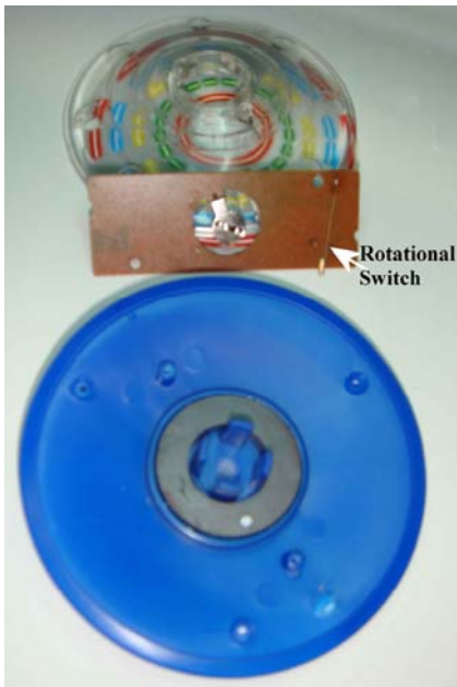
Fig. 6 – Circuit board turned over. Fig. 7 – Spinning top LEDs are turned on by the centrifugal force of rotating.
