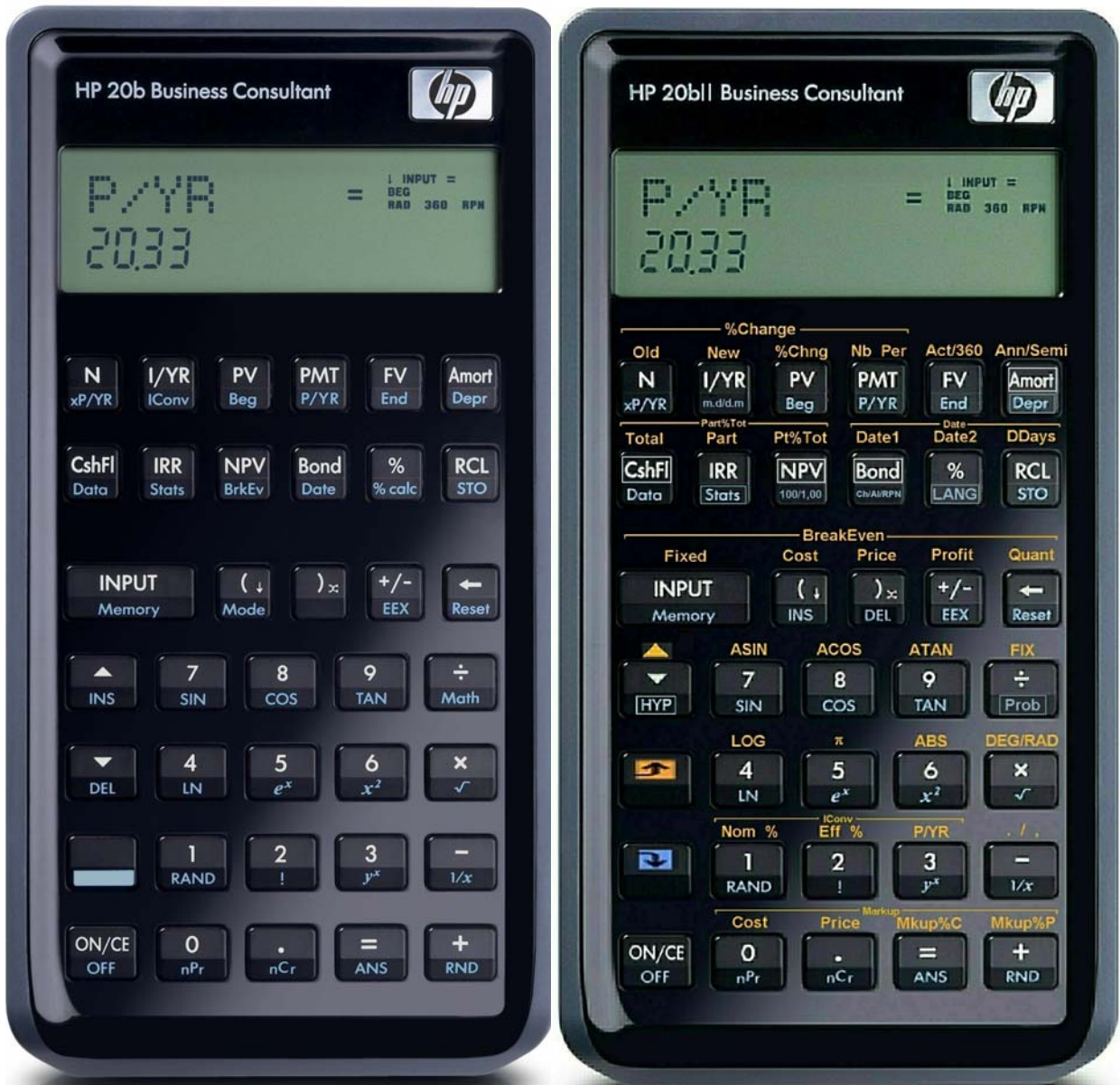
Figure 2. The HP20b (left) and a proposed “20bII” (right). Adding a second shift key enables 34 additional functions on the physical keyboard and eliminates roughly ten menus.
