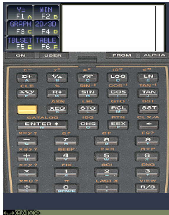
Figure 5: Image file created from scanned image of actual HP41CX calculator keyboard attached to HP49 display, to be used with HrastProgrammer's HP41 Emulator for the HP49.
