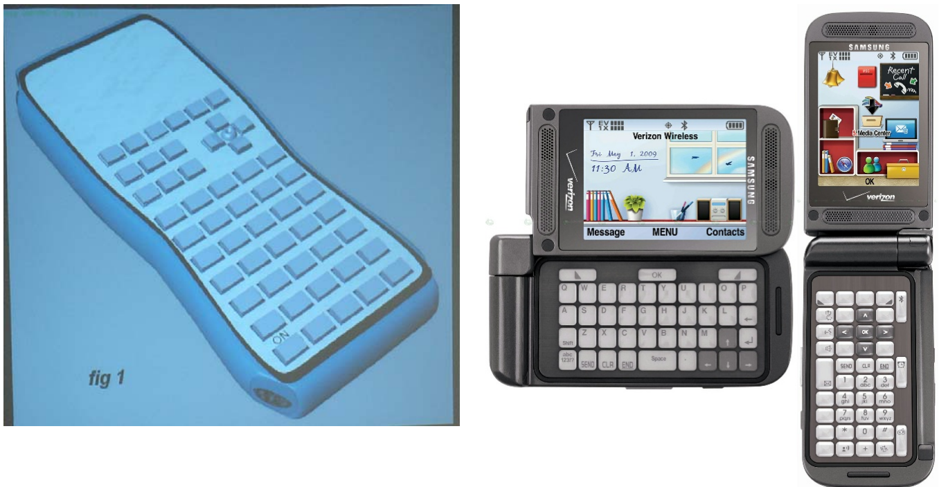
Figure 4. Left, Tim Wessman’s 2005 HP Design-A-Calculator contest winning entry with E-Ink “land” around blank real keys; Right, the Samsung Alias 2 mobile phone with E-Ink keyboard which changes with applications.
